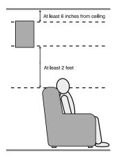
speakers should be located so that the bottom of the cabinet is at least two feet higher than the listeners' ears when the listeners are seated in the desired area.
